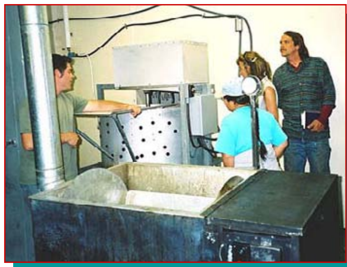
Aaron Silverman's scalding tank (foreground) and picker handle about 12 birds at a time.
